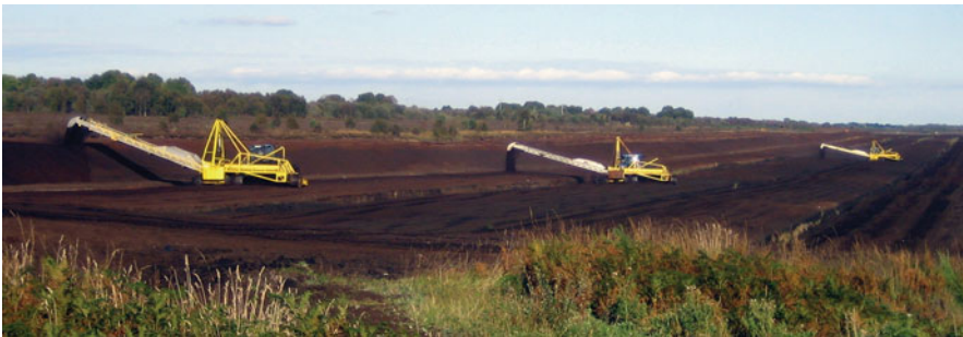
Fig. 25.5 Peat harvesting. Milled peat is collected in progressively larger piles prior to loading onto trains. (Source: Author)
